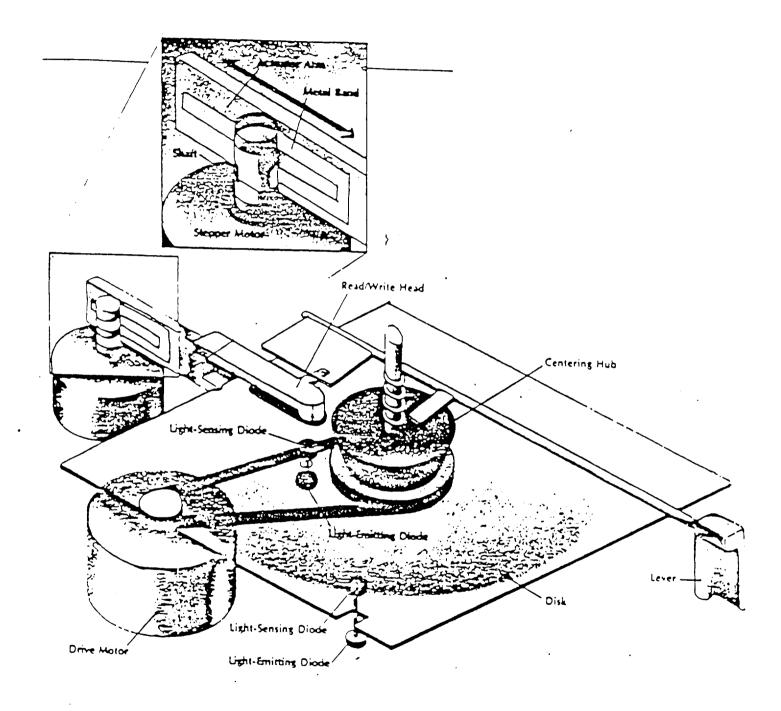
The manual lever centers the disk while closing the read/write head against the disk surface. The heads are positioned at a selected track by the combination of a DC drive motor that turns the disk and a stepper motor that moves the head assembly radially toward the disc center. Sensors, consisting of light emitting diodes (LED) and light sensing diodes verify sector position and write-protect capability.
