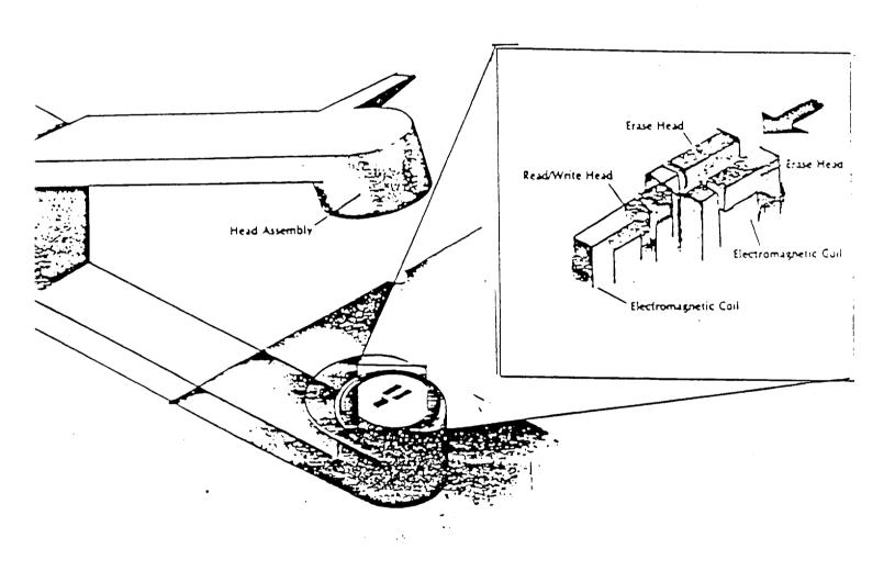
It is also noted that a read/write head is really three heads in one, the third is an erasing head. Before writing, any old information must first be erased and stray magnetic signals from the space between data tracks must be removed.
