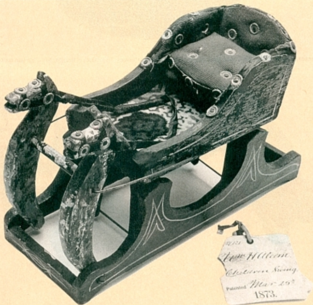
W.H. Alcorn, inventor, patent 137,121, 1873. By pulling on the reins strung between the carved horses, a child could set up an oscillating movement of the carriage's seat.
