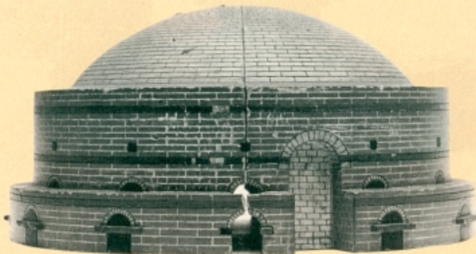
Brick-baking kiln; inventor, patent number, and date unknown. The unique design element in this kiln for baking bricks may be the way air is routed through the structure or the way the door closes.
